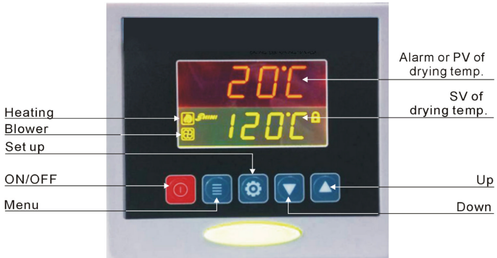
Picture 4-1: Control Panel
